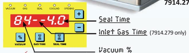
**NOTE:** Compared to the adjustment of the suction time and the visual control, the adjustment of the vacuum percentage (Vacuum%), which can be set by all Vacuweld heat sealers, guarantees maximum repeatability and precision in packaging.
