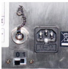
The interfacing socket, switch and power socket.
